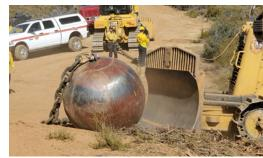
A ball and chain pulled behind a dozer crushes brush, changing fuel composition.
