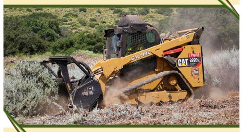
Using the skid steer with attachments, an operator can cut and masticate small and medium sized trees, remove and pile brush, and move piles of cut material to a central location for pile burning or removal.
