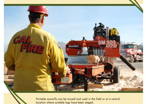
On some fuels reduction projects, there will be a few trees of good quality timber, but not enough to be economically feasible to transport to a sawmill. Portable sawmills can be used to process saw logs on-site where they can be set up next to the trees being cut. The sawn logs are used to make
