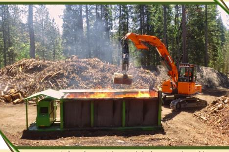
An Air Curtain Burner works by pushing high velocity air over the top of the burn chamber, creating a curtain of air which the rising smoke cannot penetrate. The unburned particulates are pushed back down into the chamber where they reburn until they are light enough to rise through the air curtain.
