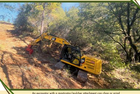
An excavator with a masticator/mulcher attachment can chop or grind vegetation into 1 - 2 inch pieces creating a break in horizontal and vertical fuel continuity. Excavators are an effective tool when creating a shaded fuel
